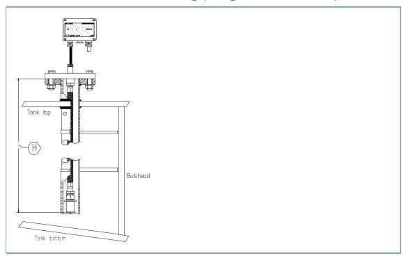
A top flange made of ASTM 316L connected to a Stainless Steel braided PTFE tube by fittings fixed to the tube by using special tools. A fitting in the opposite tube end is fixed to the transducer by means of nut and ferrules. Minimum hose bending radius is 130 mm.
